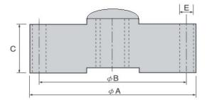
Wirop provides compression loadcells, Capacity ranges from 2.5T to 100T. The compression loadcell coupled with the Centre of Gravity solfware package. The centre of gravity can be easily found. The loadcell is made of high grade stainless steel making the loadcells are particularly suitable for rugged environments.
